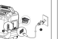
Charge the speaker until all four charging indicators light up, indicating that the battery is fully charged.
